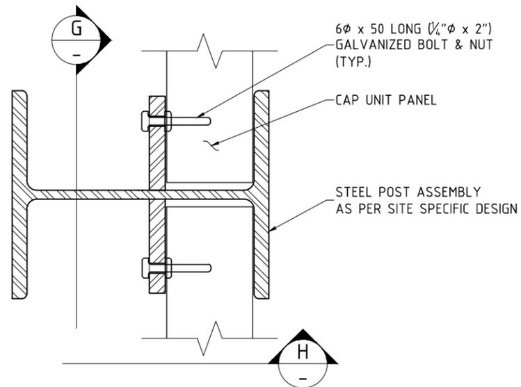
**PANEL RETENTION DETAIL - PLAN VIEW**
