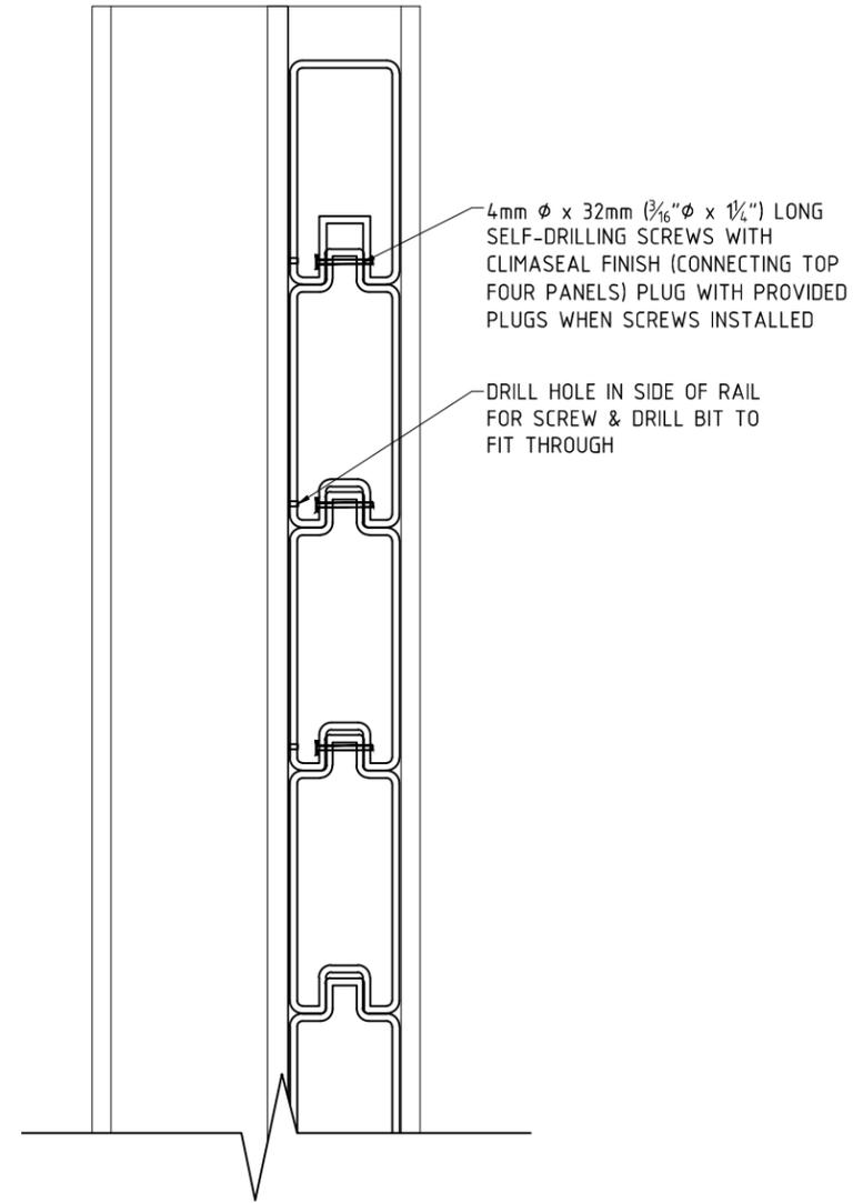
**A** SECTION - TYPICAL CROSS SECTION
