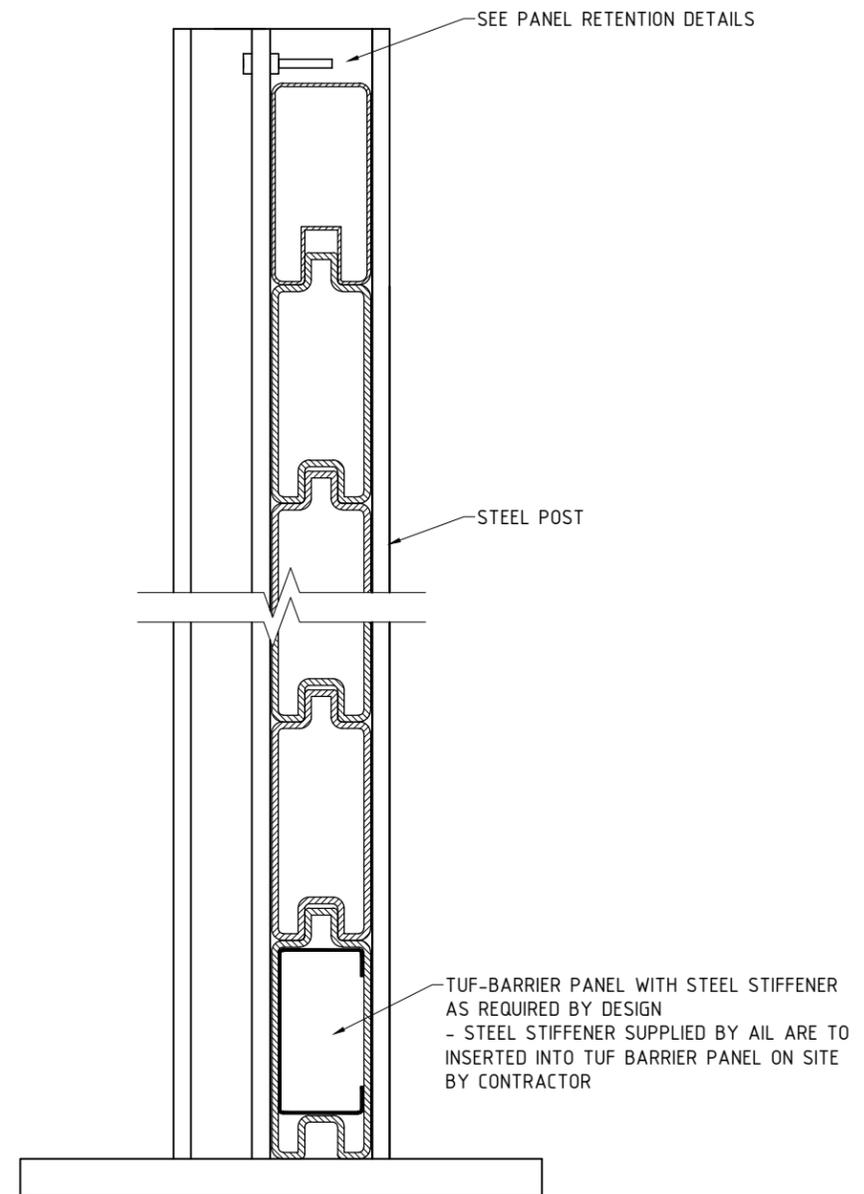
**A SECTION - TYPICAL CROSS SECTION**
