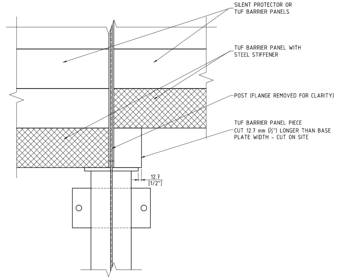
**TYPICAL STEPPED DETAIL - TYPICAL FOR STRUCTURE MOUNTED POSTS**
