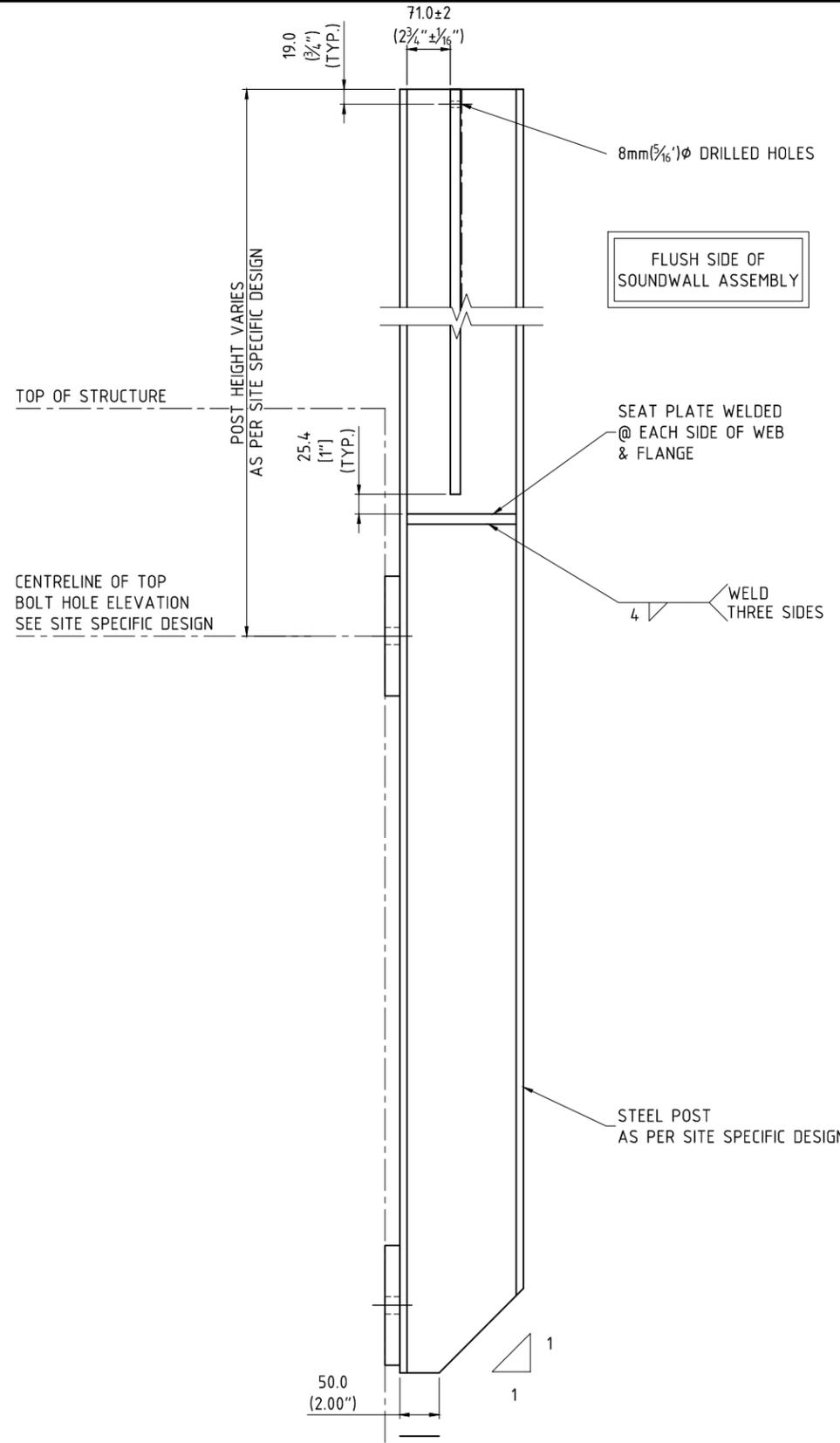
TYPICAL STRUCTURE MOUNTED STEEL POST DETAIL - SIDE VIEW
