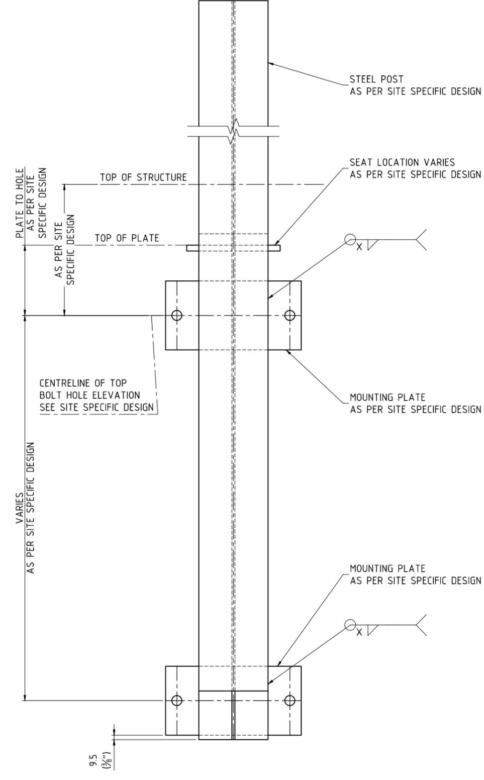
TYPICAL STRUCTURE MOUNTED STEEL POST DETAIL - FRONT VIEW
